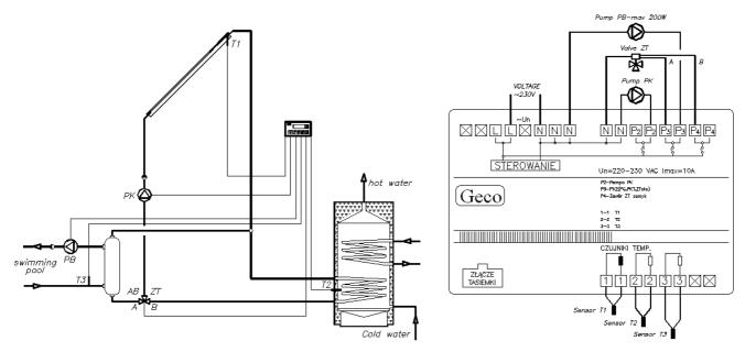
The proposed circuit operates providing for the priority of hot water, according to the principles of **1**' program version, with calibrating the valve ZT to output B. The three-way valve will be opened to output A (heating the swimming pool water) and the PK pump will be activated, if:
