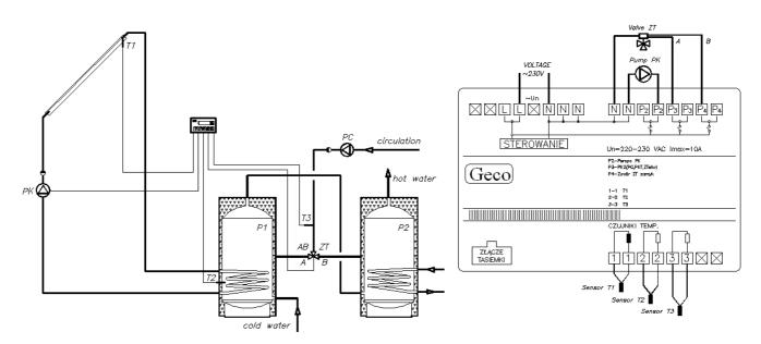
The conditions for starting PK pump are identical as in the program version '1'. The three-way valve will be opened to output A, when the difference of temperatures between the heater (T2) the return of circulation (T3) is positive and greater than the value set by the user in the parameter ' $u_3$ ' and the temperature (T3) is lower than the temperature set by the user in parameter ' $u_2$ '.
