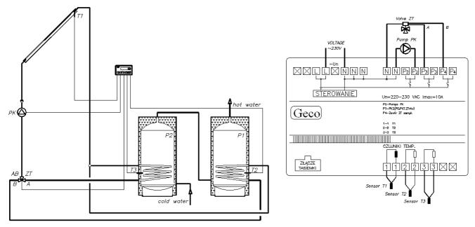
The proposed circuit operates providing for the priority of heating the water in P1 heater, according to the principles of 1' program version, with calibrating the valve ZT to output B. The three-way valve will be opened to output A (heating the water in heater P2) and the PK pump will be activated, if:
