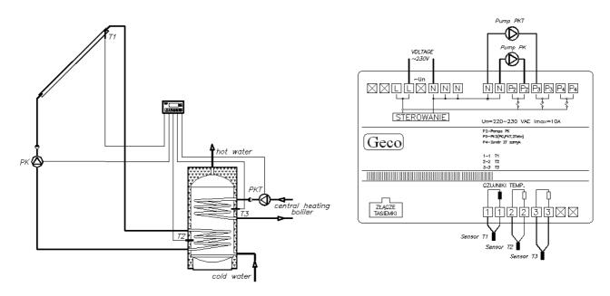
The conditions for starting PK pump are identical as in the program version '1'. PKT boiler pump will be switched on, if the temperature of sensor T3 is lower than the temperature set by the user in 'u2' parameter.
