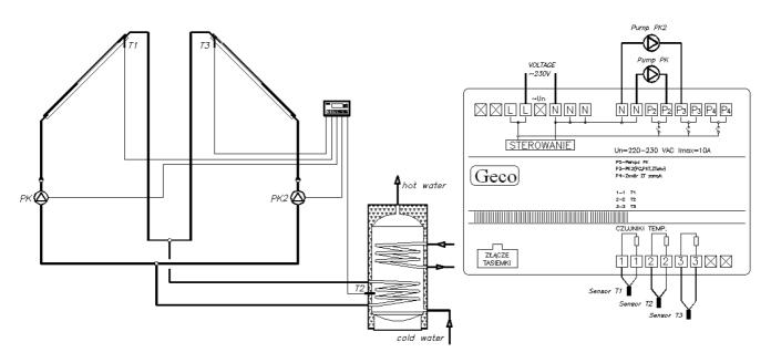
The conditions for starting PK pump are identical as in the program version '1'. The collector pump PK2 will be switched on, if the temperature difference between the second solar collector (T3) and the heater (T2) is positive and greater than the value set by the user in the parameter '**u0**' and the maximum temperature of the heater set by the user in the parameter '**u1**' is not exceeded.
